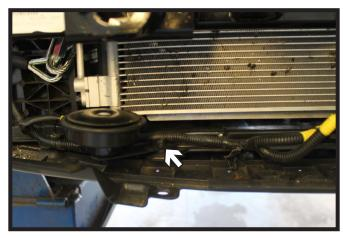
12. **Turbo Models:** Mark the bumper center brace and drill a 1/2" hole thru it to go around the electrical rod. Reinstall the brace to the bumper (left). Reinstall the horn to the existing bolt location on the left side of the intercooler (right).
