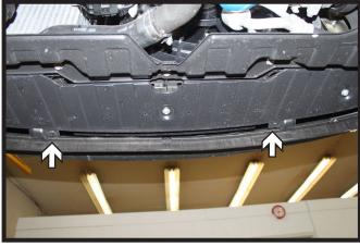
3. Using a phillips screwdriver, remove the six (6) screws from the underside of the fascia. There are two (2) on each side and two (2) in the middle.
