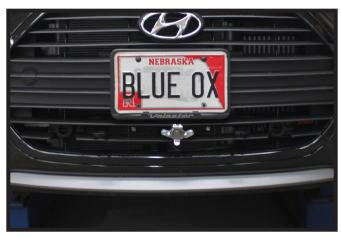
15. Hold the fascia as close to its original position, mark and trim the fascia around the convenience links and attachment tabs. Reinstall the fascia.
