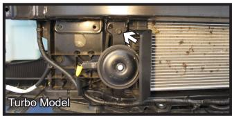
5. Using a 10MM socket, remove the screw from the horn bracket and set the horn aside.
