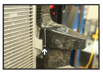
6. **Non-Turbo Models:** Trim off the lower plastic shielding as shown. Do this on both sides of the vehicle.
