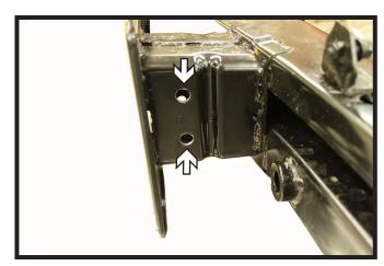
6. Using a 3/8" drill bit, ream out the existing holes on the inside of the bumper. Do this on both sides of the bumper.
