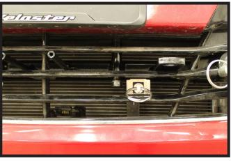
14. **Optional Breakaway:** Drill a 1/4" hole in the lower cross bar at the desired location and install the bracket & breakaway with the 1/4" hardware provided.
