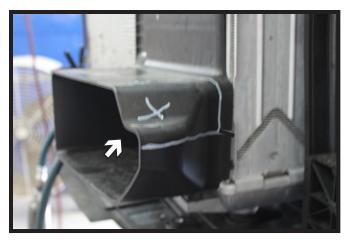
Turbo Models: Remove the vertical plastic radiator shielding (left). Do this on both sides of the vehicle.
