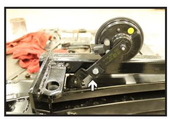
Non-Turbo Models: Reinstall the horn bracket to the bumper using the extension bracket provided.
