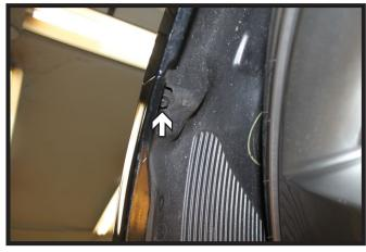
2. Using a 10MM socket, remove the screw in the wheel well at the fascia/fender joint. Do this on both sides of the vehicle.
