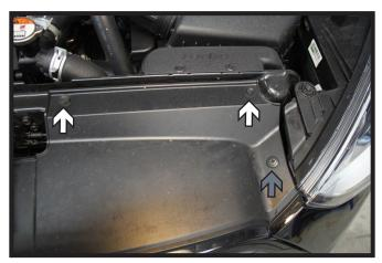
Along the top edge of the fascia, using a 10MM socket, remove the four (4) screws. There are two (2) on each side (white).
