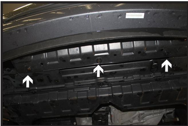
4. Using a 10MM socket, remove the three (3) screws from the middle of the fascia. **2017 Model Year:** Will need to remove five (5) screws from the bottom of the fascia.
