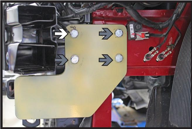
15. Using a 13/32" drill bit, drill top front hole on both sides of the vehicle thru the frame (white). Insure the baseplate remains level. Install 3/8"-16 x 1-1/4" bolts with 3/8" lock and flat washers into the holes and 3/8" nut plates in the frame. Fully tighten all hardware.
