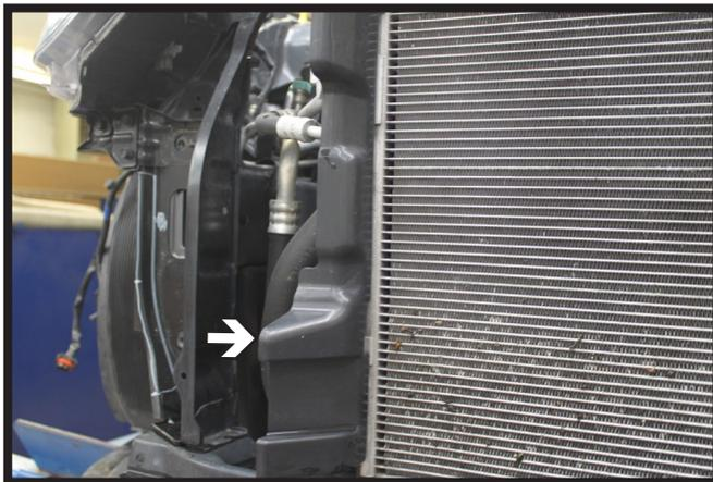
10. On the passenger side, remove the plastic shrouding next to the radiator for baseplate clearance.
