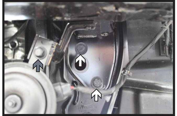
7. Using a 12MM socket, remove the two (2) bolts from bottom of bumper (white). Using a 10MM socket, remove the horn bracket bolt (gray). Do this to both sides of the vehicle. Set the bumper aside.
