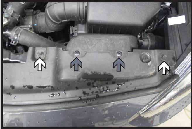
1. Using a 10MM socket, remove the four (4) screws (white) from the top of the fascia. There are two (2) on each side of the vehicle. Then remove the two (2) push pins on the driver side (gray).
