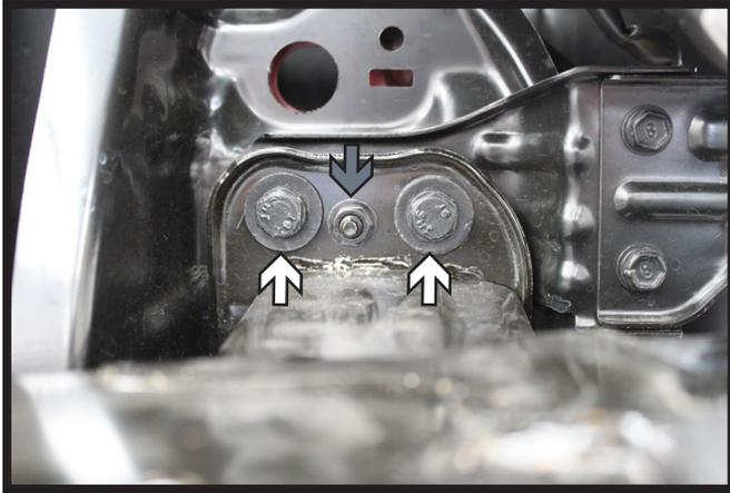
6. Using a 12MM socket, remove the two (2) bolts from top of metal bumper (white). With a 10MM socket, remove the bolt in the backside of the bumper (gray). Do this to both sides of the vehicle.
