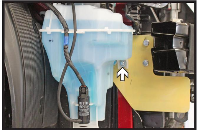
16. Remove the 6MM bolt and washer from the baseplate. Reinstall the washer reservoir, using the existing bolts in the back of the reservoir and reinstalling the 6MM bolt and washer into the baseplate. Reattach all fluid lines and electrical connections.
