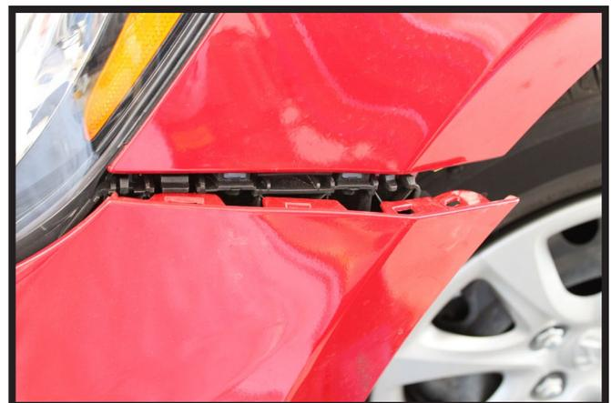
5. Lift up and pull out the corners of the fascia. Remove the fascia from the vehicle disconnecting any electrical connections and set fascia aside.
