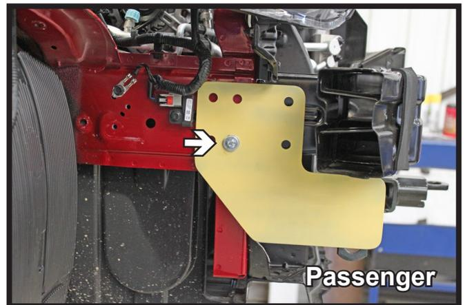
14. Mount the baseplate onto the vehicle using the existing holes on frame rails. On driver side insert a 6MM-1.00 x 45MM bolt into existing hole with 1/4" flat washer. On passenger side, insert a 6MM-1.00 30MM bolt into existing hole with 1/4" flat washer. Level the baseplate and tighten the hardware.
