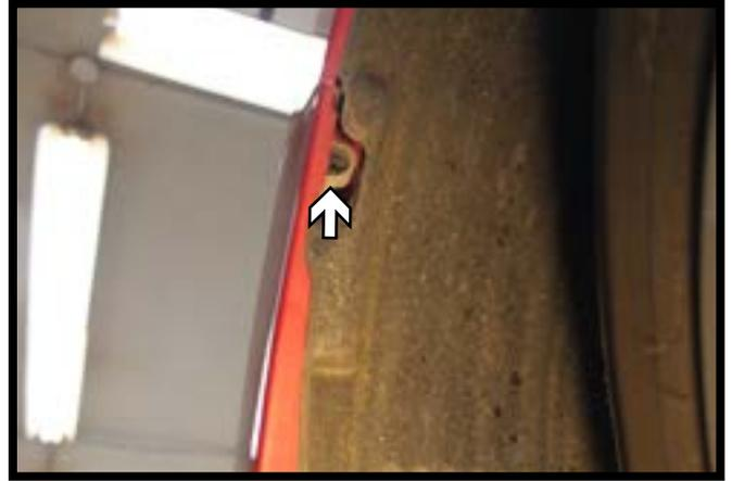
2. Using a 8MM or 10MM socket depending on the specific model of vehicle, remove the screw from the fascia/fender joint in the wheel well.
