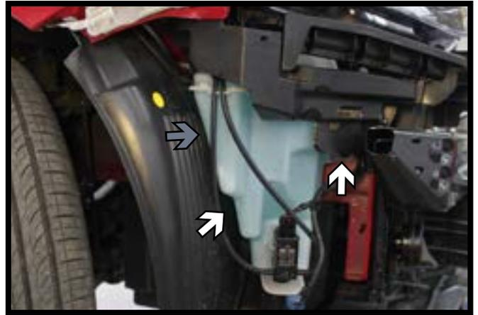
6. Using a 10MM socket, remove the two (2) screws from the washer reservoir (white). Using a phillips screwdriver, remove the upper rear screw (gray). Disconnect/plug all lines and set the reservoir aside.
