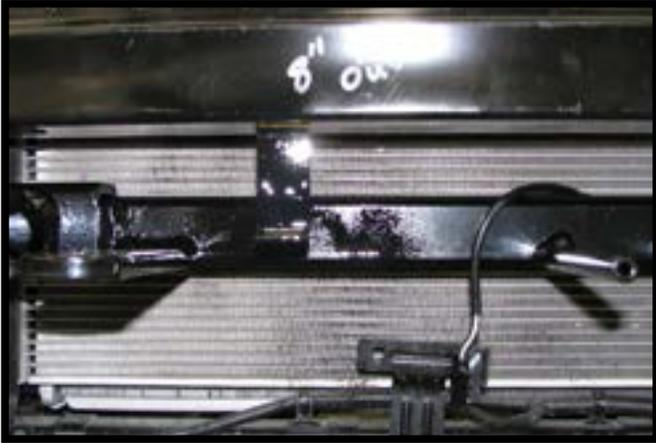
20. **Optional Breakaway:** At the desired location, attach the bracket to the vehicle with the #12 self drilling screw. Attach the breakaway to the bracket with the supplied 1/4" hardware.
