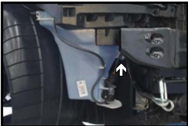
18. Reinstall the washer reservoir using the provided 6MM-1.0 x 30MM bolt on the front attachment point going thru the baseplate.
