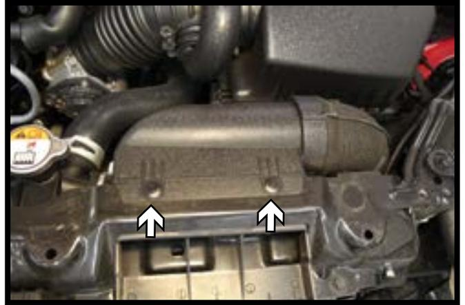
4. Remove the two (2) push pins from the intake tube and pull up to remove from the vehicle.
