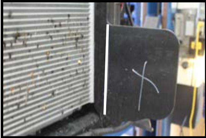
13. Trim the lower section plastic shielding back flush to the vertical edge. Do this on both sides of the vehicle.
