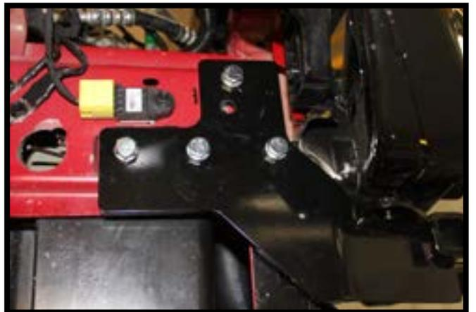
15. Install the baseplate to the frame, aligning the existing holes in the frame to the baseplate. Level and clamp in place. (It is recommended to use the existing bolts to pin the baseplate in place while leveling and clamping, then remove after baseplate bolts are installed)
