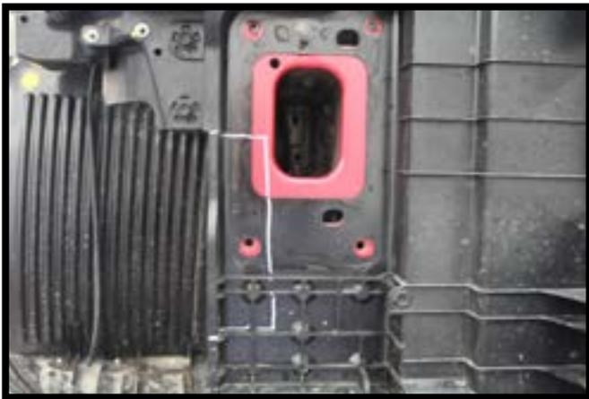
11. Using a reciprocating saw, trim the area as shown back flush to the face of the frame. Do this on both sides of the vehicle.
