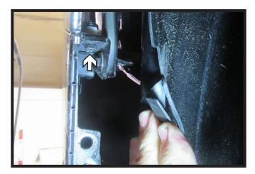
3. Pull back the wheel well liner. Using an 8MM socket, remove the one (1) bolt. Do this on both sides of the vehicle.
