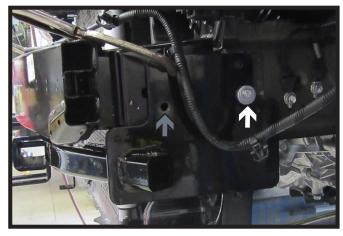
12. Slide the baseplate into place, start a 6MM bolt with hardware into the existing back hole (white). Clamp baseplate into place using a large vise grip. Using a 3/8" drill bit, drill out the front bottom hole (gray). Do this on both sides of the vehicle.
