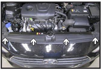
1. Using a 10MM socket, remove the four (4) bolts from the top of the fascia.
