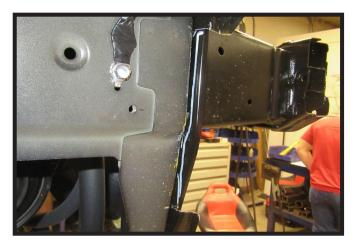
11. Hold the bumper in place and mark on the back side where the bumper over laps the frame on both sides of the vehicle. Using a reciprocating saw trim the marked areas so that the bumper is flush with the frame. Reinstall bumper and reclip wire loom to the bumper.
