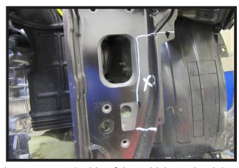
10. Using a reciprocating saw, remove the indicated areas on each side of the vehicle so that it is flush with the frame.
