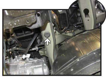
14. Remove the plug on the underside of the frame (white) and slot using a reciprocating saw to create an access hole (inset). Do this on both sides of the vehicle.
