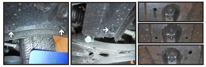
5. Remove the six (6) push pins, three (3) on each side, from the belly pan (white). Then using a 10MM socket remove the three (3) bolts along the center (gray). Remove belly pan and fascia, set aside to be reinstalled later.
