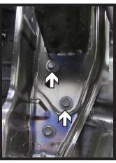
6. Using a 12MM socket, remove the four (4) bolts (white) from the bumper. Using a 10MM socket, remove the one (1) bolt (gray) on the top of the bumper. Do this on both sides of the vehicle. Unclip the wire loom from the bumper. Remove bumper and set aside to be reinstalled later.
