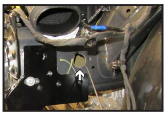
15. Using a 1-1/4" hole saw, drill out the existing hole on the side of the frame to create and access hole. Do this on both sides of the vehicle.
