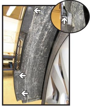
2. Remove the three (3) push pins from along the edge of the wheel well. Then using a 10MM socket remove the one (1) bolt (inset). Do this on both sides of the vehicle.
