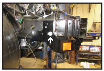
16. Slide the baseplate into place, ensure it is level, then start the one (1) 6MM bolt with hardware in the existing hole. Do this on both sides of the vehicle.
