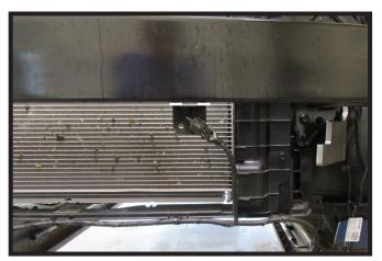
14. Using a reciprocating saw, remove the temperature sensor bracket from the bottom of the bumper. Unclip the sensor from the bracket and set aside to be repositioned later.
