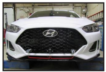
21. Hold the fascia as close to its original position, mark and trim the fascia around the convenience links and attachment tabs. Reinstall the fascia.
