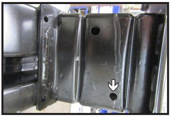
9. Using a 3/8" drill bit, drill out the small hole on the inside of the bumper. Do this on both sides of the bumper.
