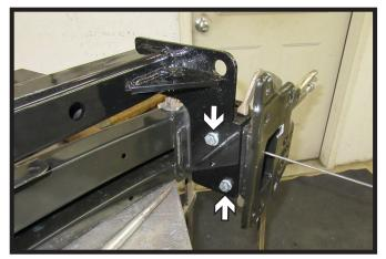
12. Install two (2) 3/8" bolts with lock washers and nut plates into the existing holes. Do this on both sides of the bumper.
