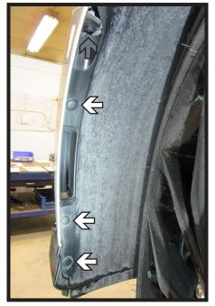
2. Remove the three (3) push pins (white) from along the edge of the wheel well. Then using a 10MM socket, remove the one (1) bolt (gray) from the fascia joint. Do this on both sides of the vehicle.
