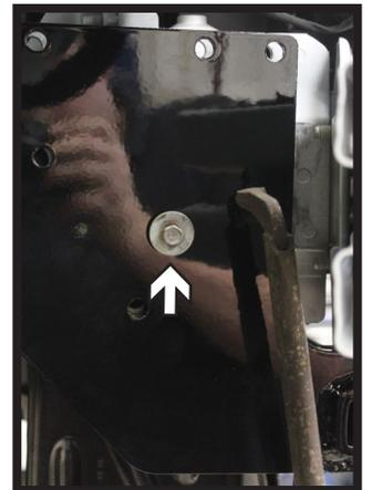
15. Slide the baseplate onto the frame, line the back of the baseplate with the mark. On the driver side pin to the existing hole in the frame (left). On the passenger side install the washer reservoir bolt into the existing hole (right). Level the baseplate and clamp it to the frame.
