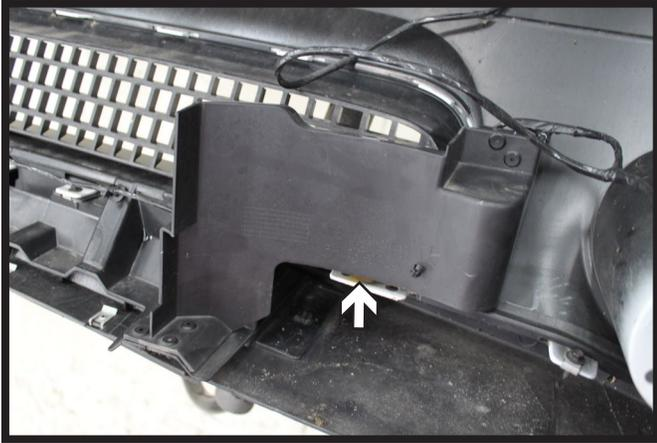
20. Before reinstalling the fascia, remove the plastic shielding from both sides by removing the plastic rivets.
