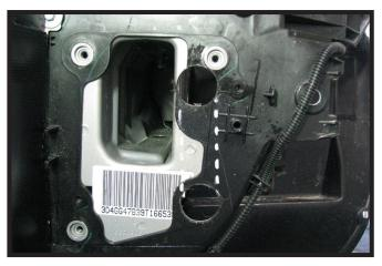
11. Using a 1-1/4" holesaw, drill out the two (2) holes. Using a reciprocating saw, connect the two (2) holes. Do this on both sides of the vehicle.
