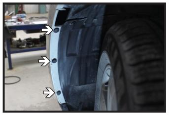
2. Remove the three (3) push pins from the wheel well. Do this on both sides of the vehicle.
