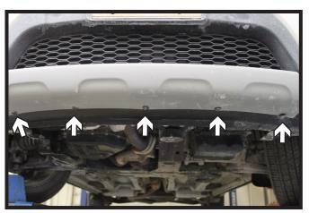
Continue along the underside of the fascia removing the five (5) push pins along the front.
