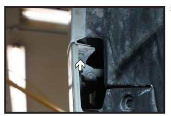
Using a 7MM socket, remove the screw from the top edge of the fascia in the wheel well. Do this on both sides of the vehicle.
