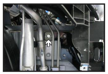
16. On the passenger side, level up the baseplate and clamp to the frame. Using a 13/32" drill bit, drill the upper left hole thru the frame. Install a 3/8"-16 x 1-1/4" bolt and lock washer into hole. From the inside of the frame install a 3/8" flat washer and 3/8"-16 lock nut onto the bolt and tighten. Drill the remaining two (2) holes and install the 3/8" fasteners.
