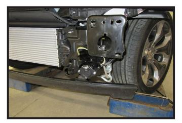
12. Attach electrical plug to the driver side baseplate using two (2) 1/4" screws.
