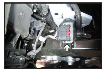
Unplug the electrical from the driver side of the vehicle. Remove the bumper/fascia and set aside to be reinstalled later.
