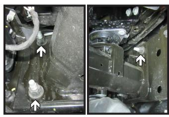
Using an 18MM socket, remove the three
