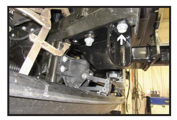
6. Slide the baseplate onto the frame and start the front 14MM existing bolt. Do not use Loctite® Red at this time. Do this on both sides of the vehicle.
