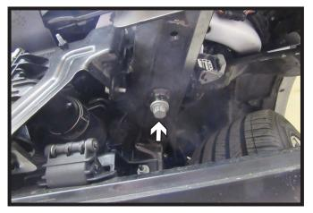
5. **Trucks with Tow Hooks:** After removing the tow hooks reinstall the back existing tow hook bolt and hardware. Do this on both sides of the vehicle.
