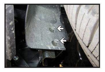
1. Using an 8MM socket, remove the three (3) bolts from the wheel well edge. Then remove the two (2) bolts from the wheel well on the inside of the tire. Do this on both sides of the vehicle.
