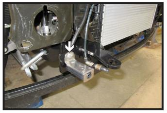
11. **Optional:** Attach breakaway switch to the passenger side baseplate using 1/4" bolt and nut.
