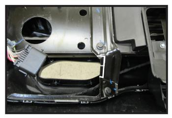
Using a reciprocating saw, remove the indicated area on the back side of the fascia to allow room for the baseplate. Do this on both sides of the fascia.
