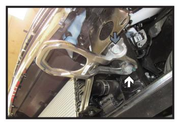
4. **Trucks with Tow Hooks:** Using an 18MM socket remove the front bolt (gray), and then using a 21MM socket remove the back bolt (white) attaching the tow hook to the frame. Do this on both sides of the vehicle. The tow hooks will not be reinstalled.
