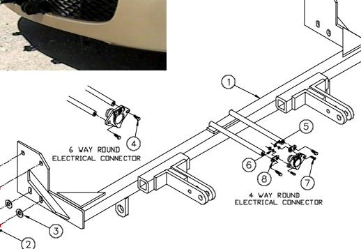
**IMPORTANT:** Use only genuine factory replacement parts on your Base Plate. Do not substitute homemade or nontypical parts. If a bolt is lost or in need of replacement, for your safety and the preservation of your Base Plate, be sure to use a replacement bolt of the same grade (Usually Grade 5, refer to parts list). Repair parts may be ordered through your nearest **Blue Ox** dealer or distributor.
