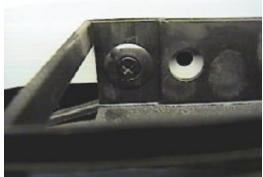
**2.** Remove the four push pins from the top side of fascia.
