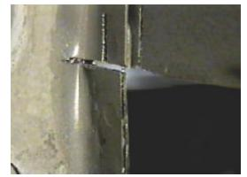
7. Remove the four metric bolts from tie down brackets with the 14MM socket, both sides. Tie down brackets will not be reinstalled. Using the hack saw, cut horizontally, the ribbing just forward of tie down bracket location, flush with frame face, and bend forward. Then make two vertical cuts 1/ 2" up from horizontal cut and bend piece forward. This will allow enough clearance for baseplate.
