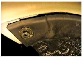
**4.** Using the 8MM socket, remove the three metric bolts on lower fascia corner, both sides.
