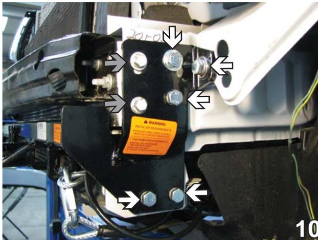
10. Align the baseplate with the seven existing holes in the frame. Insert the existing bolts (gray arrows) with Loctite into the baseplate and tighten. Use 10MM-1.5 x 40MM hex bolts with Loctite and 10MM lock washers in all the holes. In the top two also use a 10MM flat washer. Do this to both sides of the vehicle.
