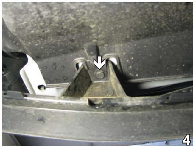
4. Remove three bolts from across the bottom corner of the fascia, using the 10mm socket. Set bolts aside to be reinstalled later.
