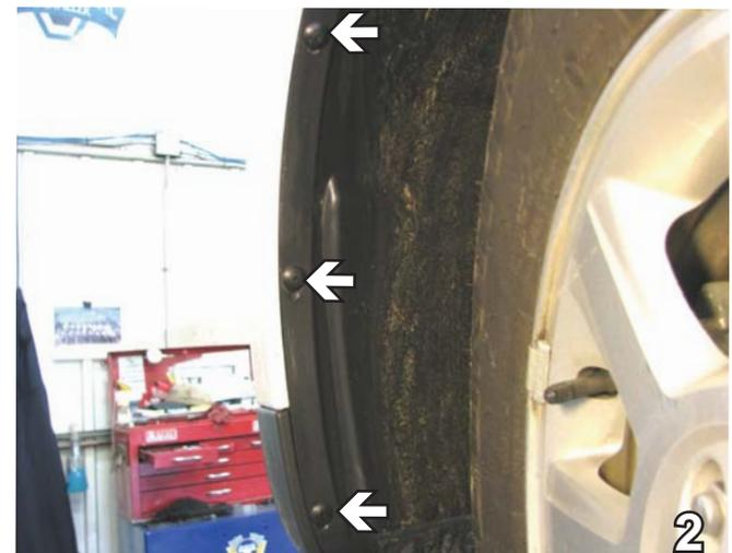
2. Just forward of the front tire, inside the wheel well, remove three Phillips push pins. Do this to both sides of the vehicle. Set push pins aside to be reinstalled later.
