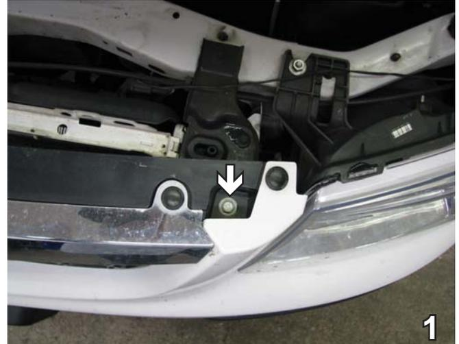
1. On the upper corner of grille, use the 10mm socket to remove one metric bolt. Do this to both sides of the vehicle. Set bolts aside to be reinstalled later.
