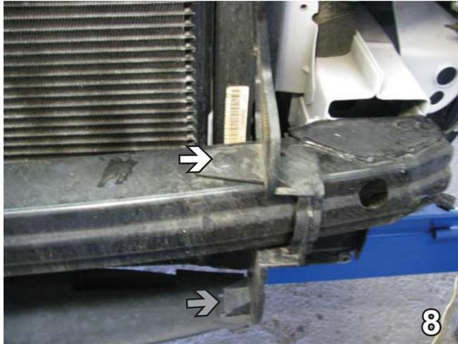
8. Using the flat screw driver, remove push pin from the piece of plastic on the outside of the bumper. Unhook the plastic from the top and the bottom (gray arrow). Do this to both sides of the vehicle. Set aside to be reinstalled later.
