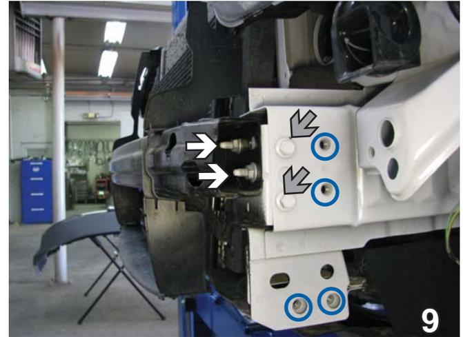
9. Remove the two nuts holding the bumper on with a 13mm socket. Do this on both sides. The bumper core is removed and not reinstalled. Set the nuts and bumper aside to reinstall later. The two bolts on each side (gray arrows) are removed with a 13mm socket and will be used to attach the baseplate. Note: Some vehicles may not have these holes (circled) with threaded inserts, see supplemental options on page 2 for hardware conversion.
