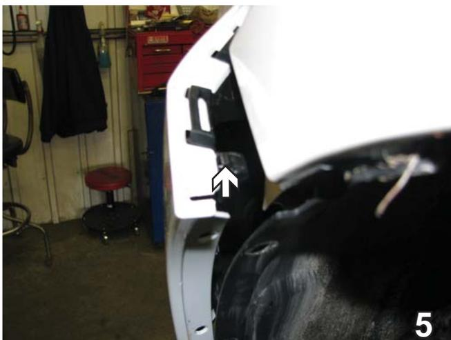
5. Reach in behind the fascia and push the clip holding the fascia down to release. Do this to both sides of the vehicle.
