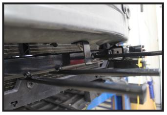
12. **Optional:** Position the breakaway bracket in the desired location. Drill a 1/4" hole into the bumper and secure the bracket to the bumper with a 1/4"-20 x 3/4" bolt and 1/4"-20 lock nut. Attach the breakaway to the bracket with a 1/4"-20 x 3/4" bolt and 1/4"-20 lock nut.
