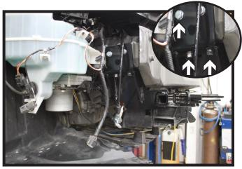
9. Using a 13/32" drill bit, drill the remaining three (3) holes on each side. There are two (2) underneath and one (1) at the rear. Remove the clamps. Install 3/8"-16 x 1-1/2" bolts with 3/8" lock washers into all of the holes with 3/8"-16 nut plates on the inside of the frame. Tighten all fasteners.
