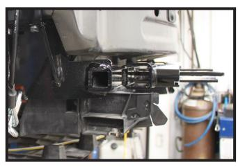
Mark and trim the air deflectors around the baseplate. Then reinstall back onto the vehicle.
