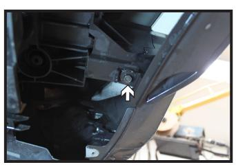
5. Using a 10MM socket, remove the screw from underside of the fascia. Do this on both sides of the vehicle. Remove the fascia from the vehicle and set aside.
