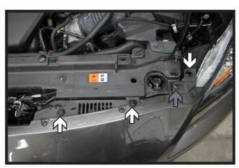
Using a Phillips screwdriver, remove the screw from the top edge of the fascia (gray). Remove the three (3) push pins (white). Do this on both sides of the vehicle.
