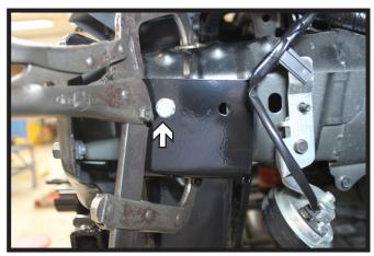
8. Using a 13/32" drill bit, drill out the front holes of baseplate on each side. Install 3/8"-16 x 1-1/2" bolts with 3/8" lock washers into the holes and 3/8"-16 nut plates on the inside of the frame. Check for level and tighten down both fasteners.
