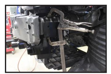
7. Slide the baseplate onto the vehicle, lining up the holes in the baseplate with the existing slots in the frame. Level and clamp the baseplate into position.
