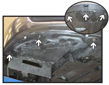
3. Using an Phillips screwdriver or 8MM socket, remove the nine (9) screws from the underside edge of the fascia. There are three (3) on each side and three (3) in the center.
