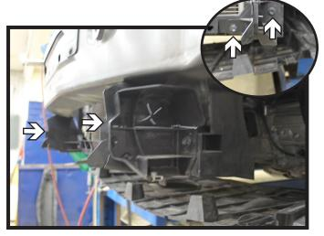
6. Using a 10MM socket, remove the two (2) screws from air deflector and set aside. Do this on both sides of the vehicle.
