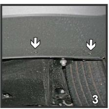
3. **MKT models:** In front underneath, using a 5.5MM socket remove seven bolts. Pull fascia corners out to the side of the vehicle, then pull forward. Set fascia and bolts aside carefully to be reinstalled later.
