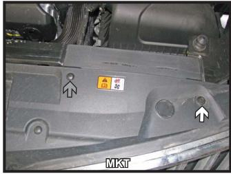
MKS models: Using a 10MM socket, remove the two (2) bolts (white arrows) from the top of the fascia on both sides of the vehicle. Use a flat screwdriver to remove the push pin in the center (grey arrow). Set bolts and push pins aside to be reinstalled later.
