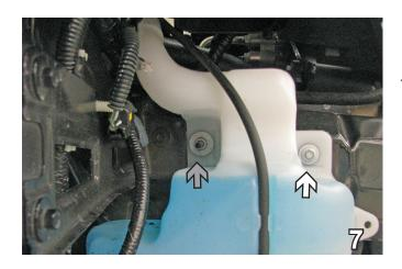
7. Continuing with the washer reservoir, use an 8MM socket to remove the top right metric bolt which will not be reinstalled. Unplug everything and completely remove. Plug the hoses to avoid losing the fluid. Set the washer reservoir aside to be reinstalled.
