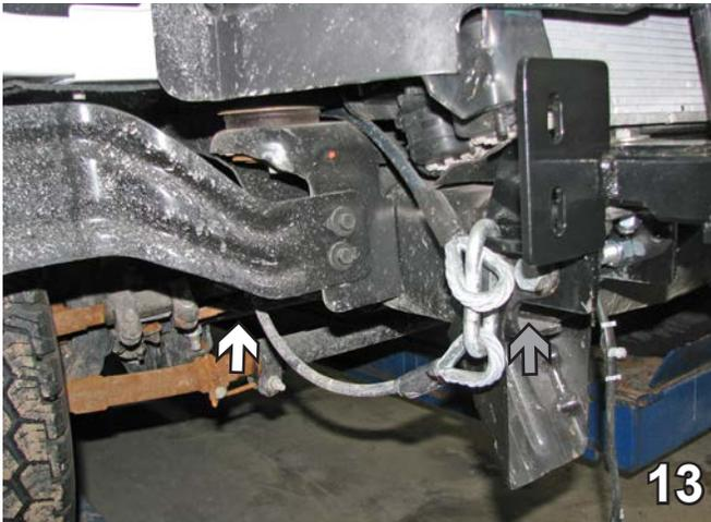
13. Attach the permanent baseplate safety cables to the provided convenience link on the baseplate. The photo shows the recommended installation of the cables to frame of vehicle. Additional options may interfere with suggested mounting; in this case, secure the cables to a solid piece of the frame as described in the General Information sheet. Be sure the safety cables do not rub against any hoses or moving parts. Do this on BOTH sides of the vehicle.
