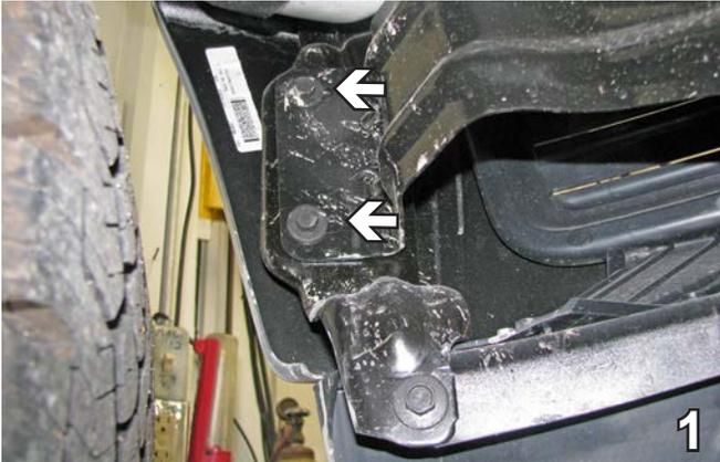
1. Using a 13MM socket, remove two metric bolts located just forward of the front tire. Do this to both sides of the vehicle. Set bolts aside to be reinstalled later.
