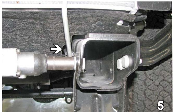
5. On the driver's side, it will be necessary to pull the Christmas tree pin from the coolant line bracket that goes into the frame in order to position the baseplate. It will be reinstalled later.
