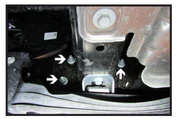
Using a 21MM socket, remove the three
