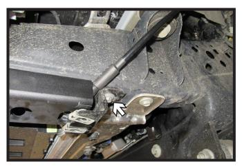
Raptor Models: Reinstall belly pan bracket before installing baseplate safety cables. Do this on both sides of the vehicle.
