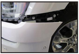
4. Remove the middle fascia piece by grabbing the edge and pulling outward. Set piece aside to be reinstalled later.
