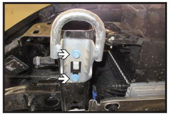
Using a 15MM socket, remove the two (2) bottom bolts from the tow hook. Remove tow hook and set aside, it will not be reinstalled. Do this on both sides of the vehicle.
