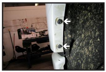
3. Using a 7MM socket or Phillips screw driver, remove the two (2) bolts from along the wheel well edge. Do this on both sides of the vehicle.
