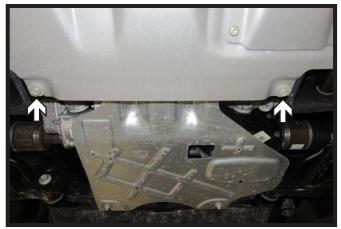
6. Using a 15MM socket, loosen the back two (2) bolts of the belly pan. Slide belly pan off the vehicle and set aside to be reinstalled later.
