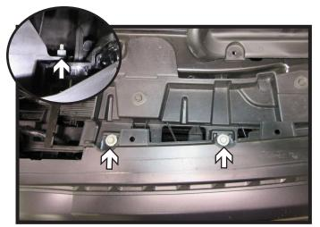
Using a 10MM socket, remove the two (2) bolts from the top of the fascia and one (1) nut (inset) from behind the head light. Do this on both sides of the vehicle.
