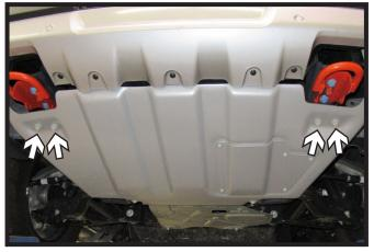
5. Using a 13MM socket, remove the four (4) bolts from the belly pan, two (2) on each side.
