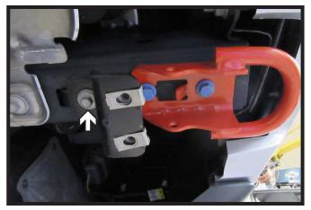
Using a 13MM socket, remove the one (1) bolt from the belly pan bracket. Remove bracket and set aside to be reinstalled later. Do this on both sides of the vehicle.
