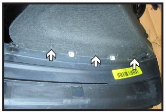
3. Using a 5.5MM socket, remove the six (6) bolts from the underside of the fascia in front of the tires.
