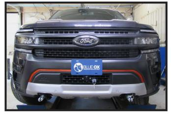
8b. **Timberline Models:** Reinstall the fascia, fascia cover, belly pan brackets, and belly pan. Reconnect sensor and all electrical connections.
