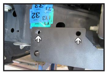
4. Using a 1/2" drill bit, drill two (2) holes in the frame using the baseplate as a template. Do this on both sides of the vehicle.
