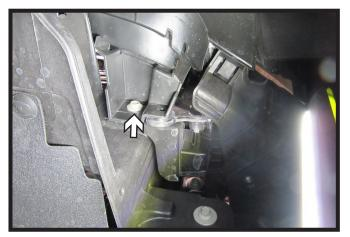
9. Using a 10MM socket, remove the one (1) bolt from underneath the vehicle in front of the radiator. Do this on both sides of the vehicle.
