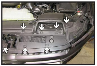
1. Remove the thirteen (13) push pins from the top fascia cover. Remove fascia cover and set aside to be reinstalled later.
