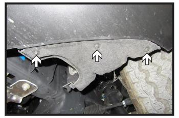
Using a 5.5MM socket, remove the three (3) bolts from the underside of the fascia in front of the tire. Do this on both sides of the vehicle.
