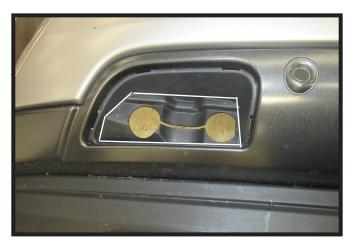
7. **Non-Timberline Models Only:** Remove the area shown to allow room for the tab and convenience link. Do this on both sides of the vehicle.
