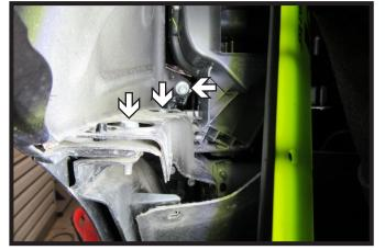
Pull back the wheel well liner. Using a 10MM socket, remove the three (3) bolts from the fascia joint. Do this on both sides of the vehicle.
