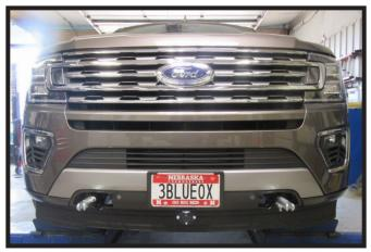
8a. **Non-Timberline Models Only:** Reinstall fascia and reconnect electrical on driver side of the vehicle.
