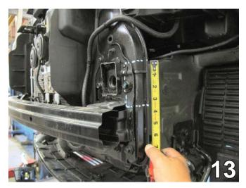
13. On the driver's side radiator support, mark and trim a section 3 1/2" high and flush with the frame rail to open the area for baseplate installation.
