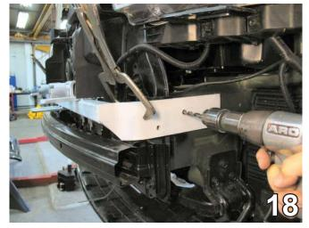
18. Slide the baseplate onto the frame through the opening in the radiator support (see steps 12 & 13). Clamp into place using the large vise grips. Using the baseplate as a template, drill three holes in the frame with the 13/32" drill bit. Do this to both sides of the vehicle, the driver's side is shown.
