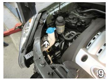
Using a 10MM socket, remove one metric bolt from the top spout of the windshield washer reservoir. Guide the windshield washer down and remove from the vehicle set aside to reinstall later. Set bolts and washer reservoir aside to be reinstalled later.
