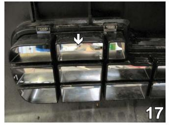
17. On upper opening, second from the grille edge, remove the horizontal grille style using the utility knife.
