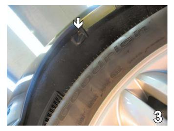
Just inside the wheel well, on the edge of the fascia, remove one metric bolt with an 8MM socket. Do this to both sides of the vehicle. Set bolts aside to be reinstalled later.
