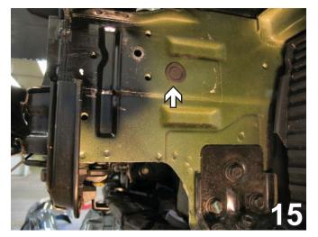
15. Remove the rubber grommet from the frame rail. Do this to both sides of the vehicle, the driver's side is shown.
