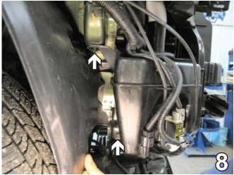
Press the wheel well cover toward the tire to expose two metric bolts to be removed using the 10MM socket. Unplug electrical connections, disconnect and plug water lines. Set bolts aside to be reinstalled later.
