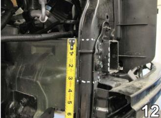
12. On the passenger's side radiator support, mark and trim a section 3 1/4" high and flush with the frame rail to open the area for baseplate installation.
