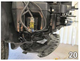
20. Reconnect electrical and water lines to windshield washer reservoir.
