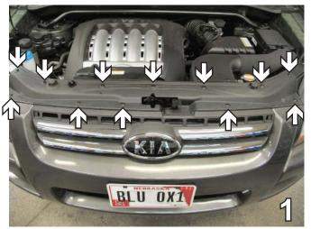
1. Remove 12 Phillips push pins from the top the fascia. Then, remove the black plastic from the top of the fascia. Set push pins aside to be reinstalled later.
