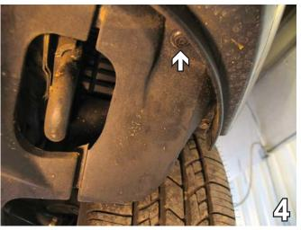
4. Just forward of the front tire, remove one Phillips push pin. Do this to both sides of the vehicle. Set aside to be reinstalled later.
