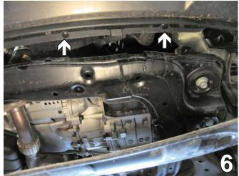
6. Remove five push pins from the bottom of the fascia, the driver's side is shown. Set push pins aside to be reinstalled later.
