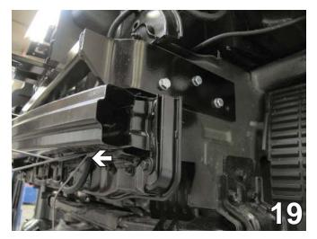
Insert three 3/8-16 nut plates through the lower bumper opening and align with drilled holes in the baseplate end plates. Insert the three 3/8-16 x 1 1/2" hex bolts and 3/8" lock washers and fasten to the nut plates. Do this to both sides of the vehicle, the driver's side is shown.
