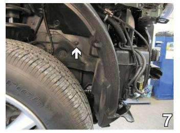
7. Remove one Phillips push pin from the wheel well cover. Do this to both sides of the vehicle. Set push pins aside to be reinstalled later.
