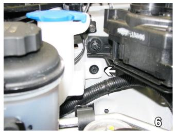
6. On the passenger side, using a 10MM socket remove one bolt from the top of the washer reservoir. Set bolt aside to be reinstalled later.
