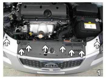
1. Using a Phillips screw driver, remove eight plastic Phillips push pins from the top of the fascia. Set push pins aside to be reinstalled later.
