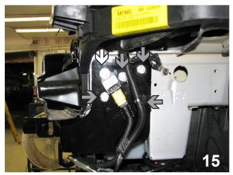
15. On the driver's side reinsert the 6MM-1 x 30MM bolt with 1/4" lock washer, 1/4" flat washer and the sensor (white arrow). Insert the remaining three 3/8"-16 x 1-1/4" bolts with 3/8" lock washers (gray arrows) and fasten to 3/8"-16 nut plates inserted into the 1-1/4" holes. Be sure to use Loctite on all the bolts. Do this on both sides of the vehicle.
