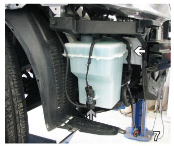
7. Using a 10MM socket, remove one bolt from the right side (white arrow) of the washer reservoir. Set the bolt aside to be reinstalled later. Unplug the electrical connection and the hose and cap the hose (gray arrow).
