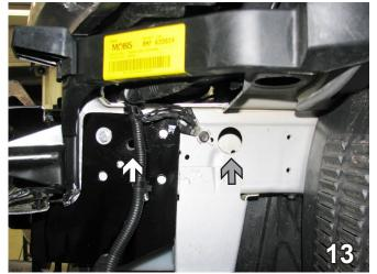
13. Using a 13/32" drill bit with the base plate as a template drill one hole (white arrow). Using a 1-1/4" hole saw, drill a hole in the frame next to the ground wires for the nut plates (gray arrow). Do this on both sides of the vehicle. Be sure to install only one bolt assembly per side to stabilize baseplate before drilling the remaining holes.
