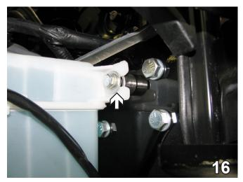
16. On the passenger side, insert the three 3/8"-16 x 1-1/4" bolts with 3/8" lock washers and fasten to 3/8"-16 nut plates inserted into the 1-1/4" holes. Be sure to use Loctite on all the bolts. Reattach the washer reservoir using the existing bolts and a 6MM-1 x 45MM bolt with 1/4" lock washer, 1/4" flat washer and 1/2" spacer tube into the hole shown.
