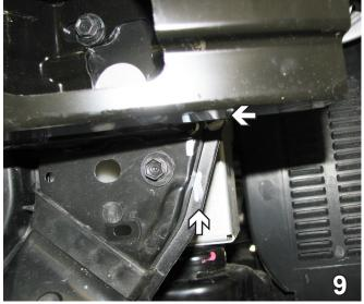
9. Trim flush with the bottom of the frame and in until even with the side of the frame. Do this to both sides of the vehicle.
