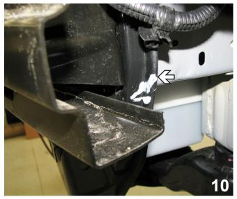
10. Go up 1/2" from where the cut started flush with the bottom of the frame. Cut out a v notch to the point of intersection with the side of the frame. Do this to both sides of the vehicle.
