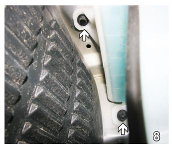
8. Using a 10MM socket on the left side of the washer reservoir remove two bolts. Set bolts and reservoir aside to be reinstalled later.
