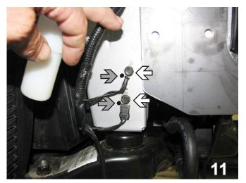
Loosen the ground wires (white arrows). Flatten the pins (gray arrows) and turn the wires to a vertical position. Do this on both sides of the vehicle.
