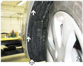
2. Using an 8MM socket, remove three bolts forward of the front tire on the wheel well. Do this to both sides of the vehicle. Set push pins aside to be reinstalled later.
