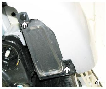
4. Underneath the fascia in the corner remove the two plastic push pins. Do this to both sides of the vehicle. Set push pins aside to be reinstalled later.
