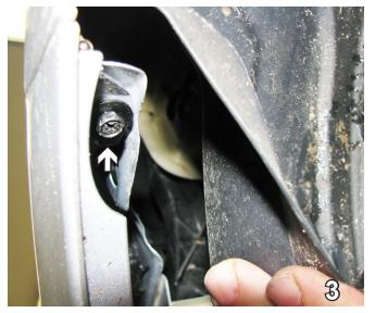
Pull the plastic wheel well cover back, using an 8MM socket remove the bolt underneath. Do this to both sides of the vehicle. Set the bolts aside to be reinstalled later.
