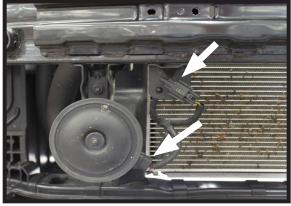
6. Unplug the horn and temperature sensor. They will be repositioned after the baseplate has been completely installed.
