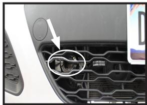
14. After the front fascia has been reinstalled trim the grill to allow ample room for the attachment tabs. Do this on both sides.
