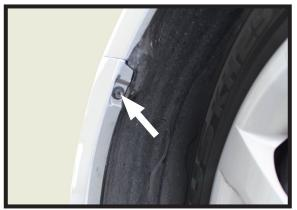
3. On the front tire wheel well remove the bolt using a 10MM socket. Do this on both sides.
