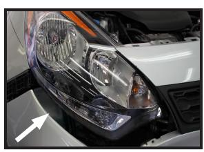
5. Pull the front fascia away from the front of the vehicle. Gently pry the fascia away from under the headlight area.
