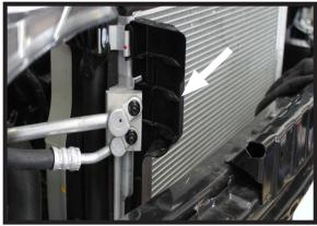
8. On the passenger side <u>ONLY</u> there is a plastic tab. Remove this tab by pulling upward. It will not be reinstalled.
