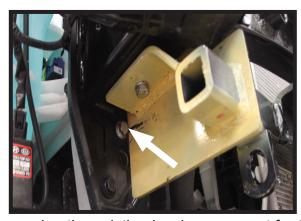
12. Reattach the bumper frame using the existing hardware except for the top bolt on the bottom section of the bumper bracket. The supplied 8MM bolt replaces the bolt that was removed as the attached washer would not allow the bolt to be started. Do this on both sides of the vehicle.
