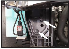
7. To remove the front bumper, unclip the wiring harness and place it out of the way. Next, remove the bumper using a 12MM socket for the two (2) outer bolts and 10MM socket for the center bolt on the top of the bumper frame bracket. On the bottom of the bracket there are two (2) 12MM bolts that need to be removed. Do this on both sides of the vehicle.
