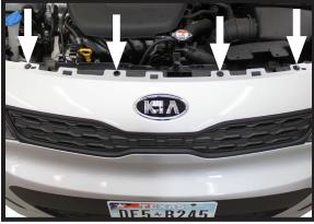
2. Once the push pins have been removed, pop the plastic covers off. Underneath the covers there are four (4) additional push pins, two (2) per side, that must be removed.
