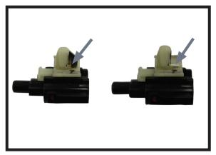
13. The temperature sensor will need to be relocated from the slot to the adjacent hole. In order for the sensor to fit you must trim the attachment bracket. The horn will be placed in the slot that the temperature sensor was originally located in.
