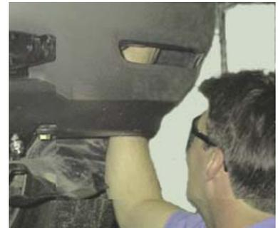
7. Feed the 3/8" bolt plate with wire (Item 2) through the lower channel of the metal bumper and into the drilled hole. Bolt the baseplate to metal bumper, hand tighten only.
