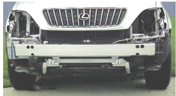
9. Bolt the braces (Items 10) to the outside holes on the baseplate (Item 1) using 1/2-13 x 1 1/2" Hex bolt and hardware (Items 8, 4 and 5). As shown in diagram on page 2. Thread nuts slightly so braces are loose.
