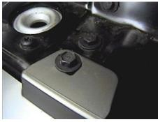
2003-'04 Models: Remove the three metric bolts from top side of upper grill using the 10MM socket. 2005 Model: Requires a 7MM socket. Pull grill forward and up, disconnect temperature sensor and set grill aside.
