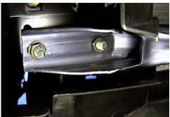
7. Remove the four metric nuts from cross tube, just below metal bumper, with the 16MM socket and two metric bolts from the center braces with the 10MM socket, set tubing aside. Tubing will not be reinstalled. Also remove the two metric nuts just above the metric nuts on cross tube seen in the photo, both sides. Some 2005 Models may not have this cross tube to remove.
