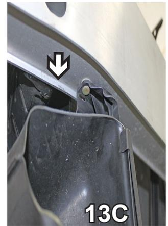
13. To remove the air baffles, with a 10MM socket, in front of the tire, remove bolt (13A), under the air baffle, remove two (2) bolts (13B) and unsnap the air baffle at the bottom of the metal bumper (13C). Do this on both sides. Pull down air baffles to remove and set aside air baffles and bolts to be reinstalled later.
