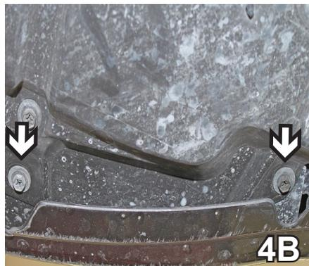
4. To remove the bumper, with a 10MM socket, remove eight (8) bolts from the underside of the fascia. Set bolts and bumper aside to be reinstalled later.
