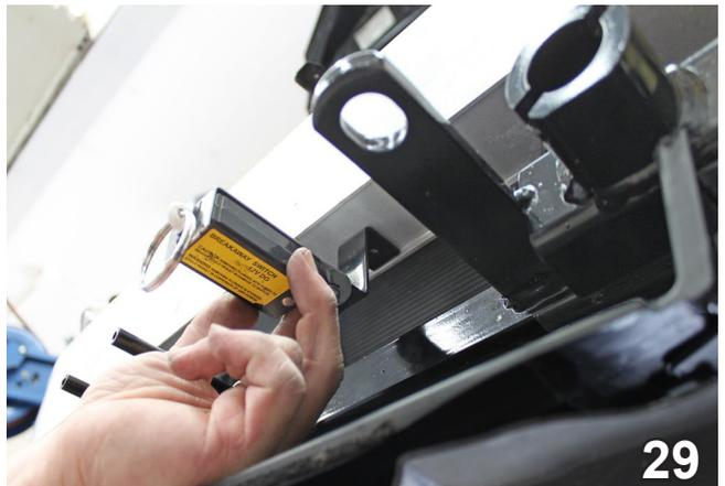
29. **Optional:** Mount the breakaway bracket to the bottom of the metal bumper, all the way back to the bottom ridge of the bumper. Position it half-way between the electrical rods and the convenience link. Install using 1/4"-20 x 3/4" hex bolt, 1/4"-20 hex nylon nut, and #10-16 x 1" self-drilling screw.
