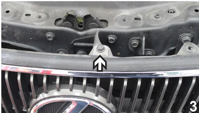
3. Just above the vehicle's emblem, remove bolt from vehicle support using a 10MM socket. Set bolt aside to be reinstalled later.
