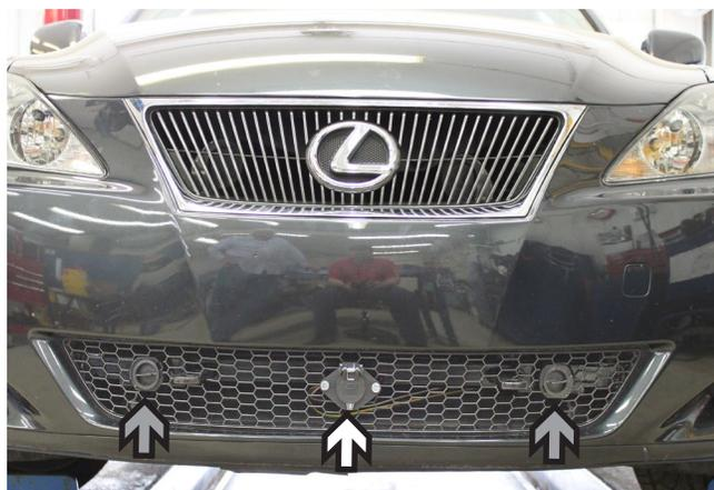
30. Reinstall fog lights and connect sensor back onto fascia. Align the fascia to its original position and trim the opening for the attachment tabs with diagonal cutters (gray arrows). Do this on both sides of the vehicle.
