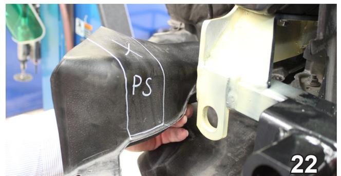
22. Before reinstallation of air baffle, hold air baffle as close to original position as possible. Mark and trim as necessary on air baffle to accommodate baseplate installation. Reinstall air baffle using existing bolts and tighten. Do this on both sides.
