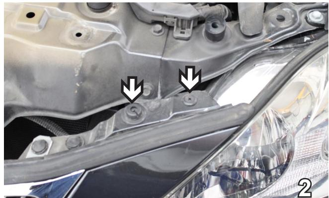
2. On top of the fascia, inside of the headlight, remove Phillips screw and pushpin. Do this on both sides. Set push pins and screws aside to be reinstalled later.
