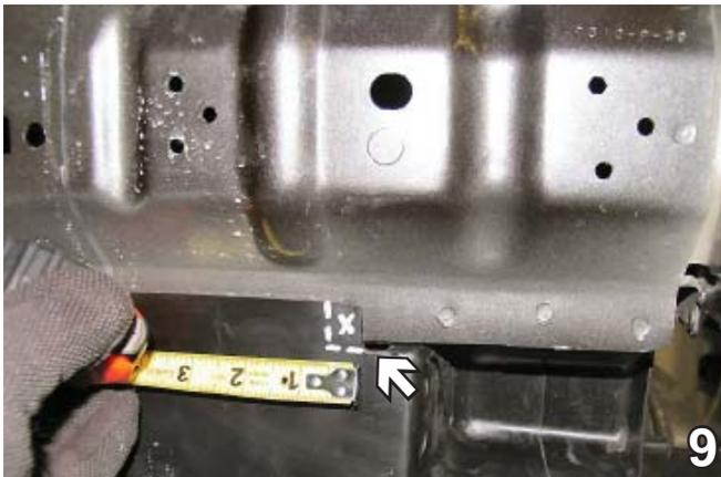
9. Mark plastic 1/2" back from front edge, cut and remove on both sides as shown in photo (photo of passenger's side).
