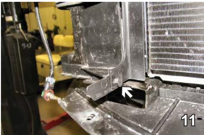
11. Remove one christmas tree push pin from lower air dam, just below metal bumper, both sides. Turn air dam in to lay flat against radiator and lift up to remove, both sides.
