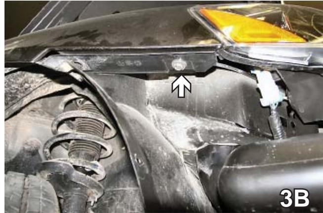
3. Using the 10MM socket, remove the back metric bolt from corner of fascia, just above front tire (left photo) and loosen the front metric bolt on the inside of wheel well, both sides (right photo shows passenger's side location with fascia off).
