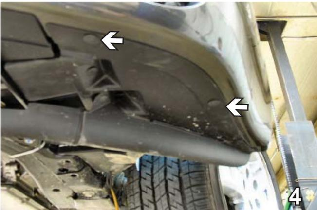
4. Remove the two push pins on lower edge of fascia, just forward of the front tire, both sides.
