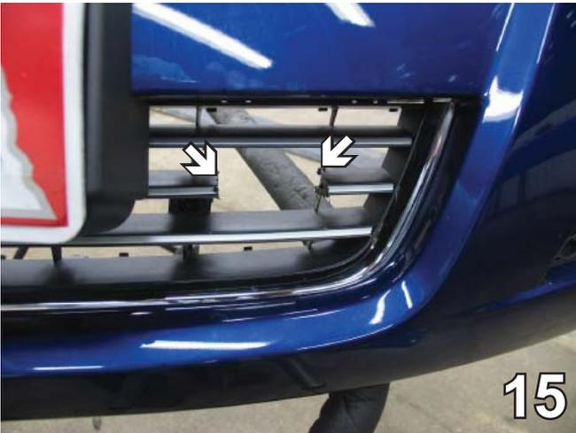
15. Using the hack saw blade, cut out the fascia middle horizontal rib to the outside of the sensor. Remove the whole piece to open the area up for baseplate installation. Do this on both sides of the vehicle.
