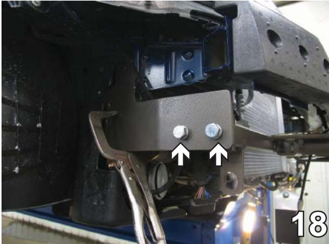
18. Loosely bolt the baseplate cross member piece to the end plates with 1/2" x 1 1/4" hex bolts and 1/2" lock washers. Be sure it is level with the vehicle and clamp to the passenger's side.
