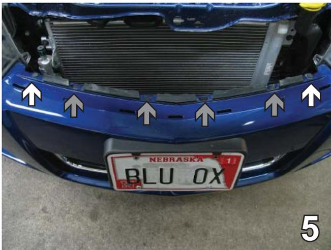
5. Remove two push pins (white arrows) from each side of the front of the fascia. Set push pins aside to be reinstalled later. Push down on the four tabs (gray arrows) across the front as the fascia is being removed. Pull fascia's upper corners out to the side of the vehicle and straight forward. Set the fascia aside carefully to be reinstalled later.
