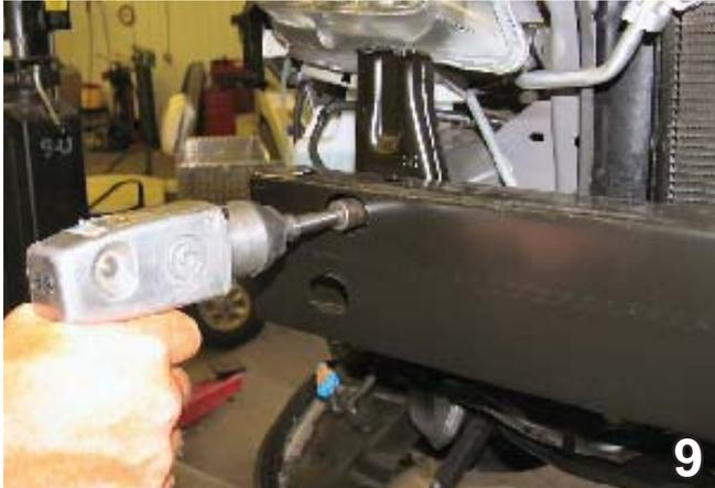
9. **ALL MODELS:** Using a 14MM socket, remove four metric bolts from metal bumper and set aside for later reinstallation.
