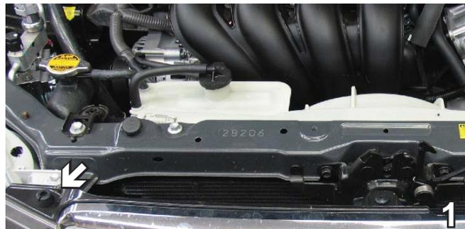
1. **2005-07 MODELS:** Using the Phillips screw driver, remove the Phillips screw from rubber bumper, do this to both sides and set rubber bumper aside for later reinstallation.
