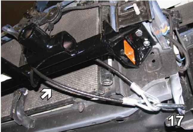
17. **2008 MATRIX:** Attach the permanent baseplate safety cables to a solid piece of the vehicle's frame as in above photos or as close to as possible.
