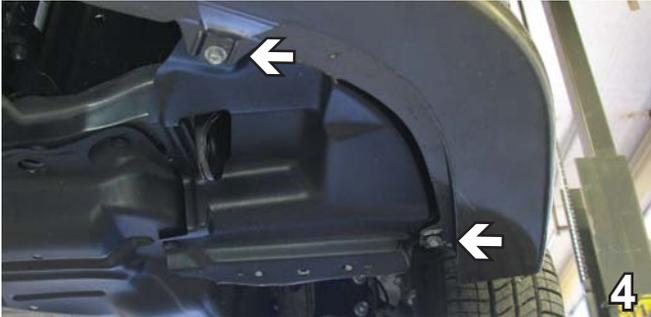
4. **ALL MODELS:** Using a 10MM socket, remove two metric bolts just forward of front tire. Do this to both sides and set aside bolts for later reinstallation.
