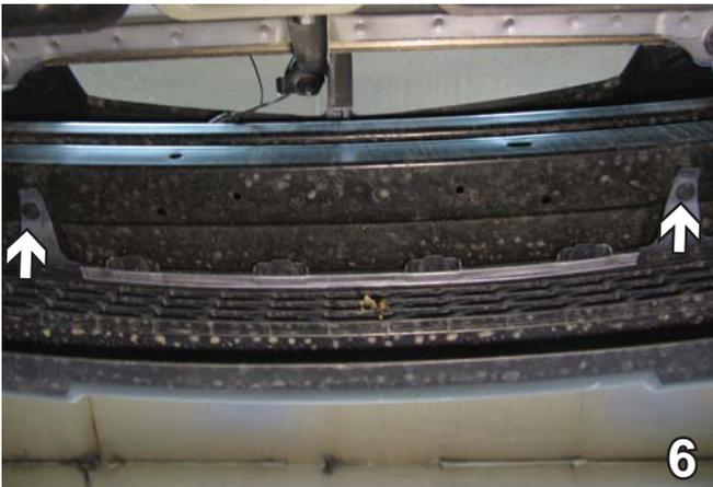
6. **2008 MATRIX:** Underneath the bumper, remove two push pins with a flat screw driver. Set aside for later reinstallation.
