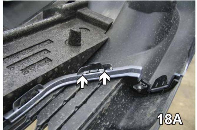
18A. **2008 MATRIX:** On the inside of the fascia, using the utility knife trim off the tab as shown. Do this on both sides.
