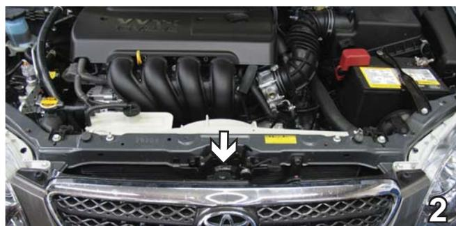
2. **2005-07 MODELS:** Remove push pin from top edge of fascia just below hood latch and set aside for reinstallation later.
