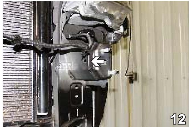
12. **ALL MODELS:** Slide baseplate up between frame rails to align with existing hole and clamp to the bottom of frame with vise grips on both sides.
