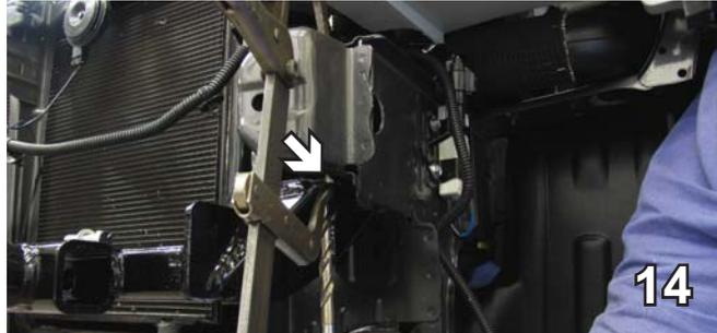
14. **ALL MODELS:** Using the baseplate as a template, drill two holes into bottom of frame with 13/32" drill bit, both sides. Insert nut plates into 1 1/4" hole on frame rail to align with drilled holes, tighten 3/8" hex bolts and lock washer with 9/16" socket on both sides.
