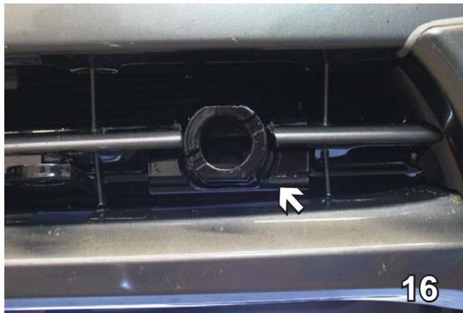
16. **2005-07 MODELS:** Hold fascia as close to its original position as possible, mark and cut grill with utility knife to allow baseplate receivers to come through. Plug in fog lights in applicable on back side of fascia and reinstall fascia.
