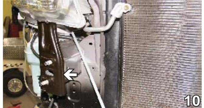
10. **ALL MODELS:** Remove bumper bracket from both sides and set aside.
