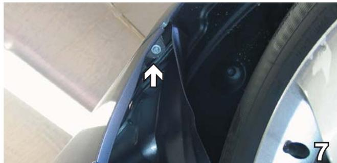
7. **ALL MODELS:** Remove metric bolt just forward the front tire on upper corner of fascia and inside of wheel well, using a 10MM socket. Do this to both sides. Pull fascia forward, unplug electrical connection to fog lights, and carefully set aside for reinstallation later.
