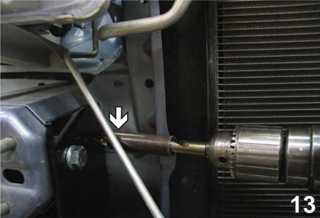
13. **ALL MODELS:** Using the baseplate as a template, drill both holes in the side of frame rail with a 17/32" drill bit. Do this to both sides. Insert nut plates into 1 1/4" drilled hole on outer side of frame rail to align with drilled holes. Tighten the 1/2" hex bolts and lock washer with the 3/4" socket into nut plates. Do this to both sides.
