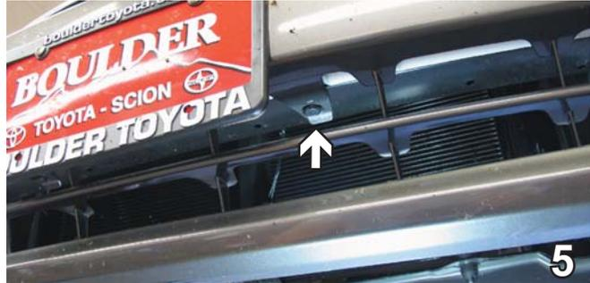
5. **2005-07 MODELS:** Behind fascia on bottom of metal bumper, are two push pins to remove from fascia's tabs. Remove with flat screw driver and set aside for later reinstallation.
