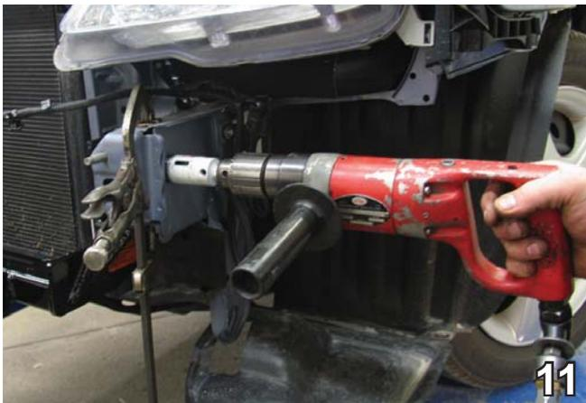
11. **ALL MODELS:** Drill a hole in the frame rail using the 1 1/4" hole saw on both sides. This hole will allow installer to insert nut plates inside of frame rail in steps 13 and 14.
