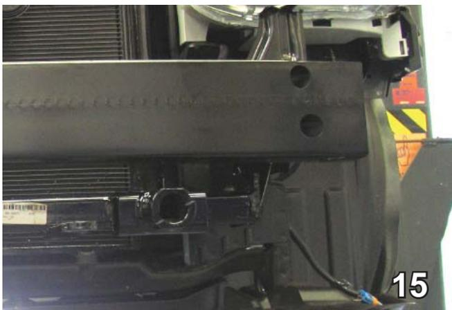
15. **ALL MODELS:** Reinstall bumper bracket, metal bumper and styrofoam. Be sure to reattach wire loom to top of bumper.
