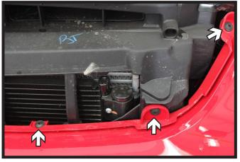
2. Using a T25 Torx, remove the six (6) screws at the top of the fascia. There are three (3) on each side.
