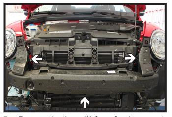
7. Remove the three (3) foam fascia support pieces. DO NOT discard, these will be reinstalled later.
