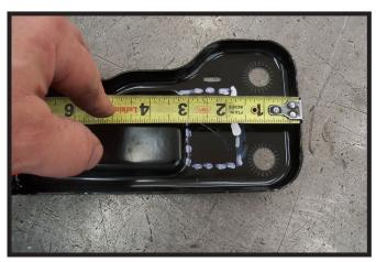
13. Cut a opening in the brace, approximately 1-1/2" down from the top down to the rib and approximately 3/4" from the sides. Do this on both braces.
