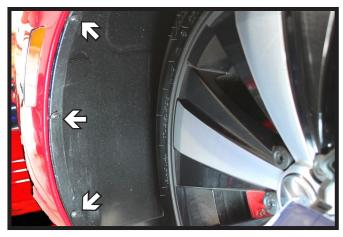
3. In the wheel well, use a T25 Torx to remove the three (3) screws. Do this to both sides of the vehicle.
