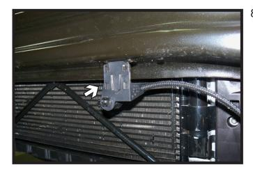
3. Remove the air temperature sensor from the bumper and set aside.
