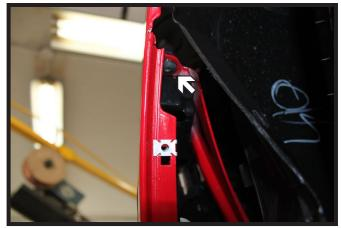
4. Behind the wheel well cover remove the one (1) upper fascia screw with a T25 Torx. Do this to both sides of the vehicle.
