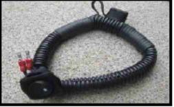
the "towed" vehicle. Confirm that the pins on the Fuse ByPass Switch wires match the pin sizes on the fuse you removed. You must have the correct fuse wire ends for your fuse box. If your vehicle is equipped with a ATM Micro Mini fuse, a ATM Mini fuse of the same rating as the OEM will need to be installed into the ATM Mini Fuse Bypass Switch holder.
