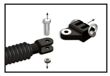
Using a 3/4" socket and wrench, remove the existing 1/2"-13 bolt and 1/2"-13 jam nut from the tow bar leg. Remove the existing lug and washers from the tow bar leg. Do this on both tow bar legs.
