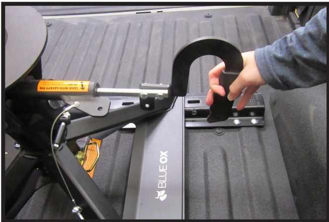
3. Turn handle clockwise till in the open position as shown. Handle will remain in this position until hook-up. Note: Verify that the handle is in the locked position before reinstalling locking pin.
