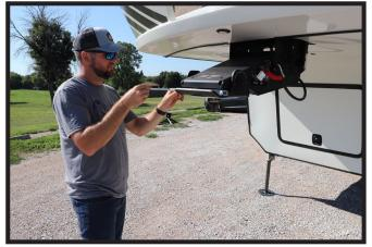
1. Place one (1) of the lockout plates behind the front lip and against the front of the pin box.
