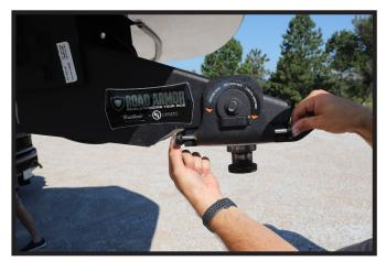
2. Insert one (1) carriage bolt into each side of the front plate. Feed bolt between pin box and pivot head.
