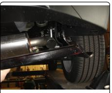
4. Torque 7/16" hardware to 59 lb-ft. Raise exhaust back into position and reinstall panel removed in Step 1.
