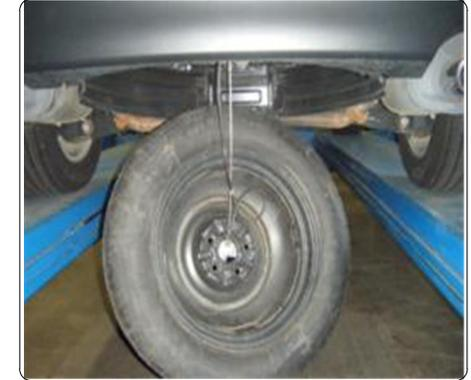
2. Fishwire 1/2" carriage bolts and CM-SP12 spacers into position through end of vehicle bumper beam.
