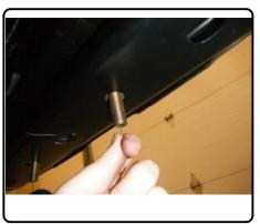
Raise hitch into position between bumper mount plates and align slots in hitch with existing vehicle weldnuts in the frame rails. Install (4) M12-1.25 hex bolts and (4) 1/2" conical toothed washers into existing weldnuts, as shown.
