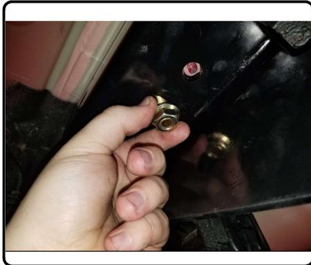
5. Install (4) M10-1.25 hex bolts and (4) conical tooth washers, (2) on each side of the hitch.
