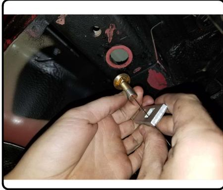
4. Raise hitch into position and feed fishwires through center hole on the hitch. Remove fishwires and loosely secure with 7/16" hex flange nuts.
