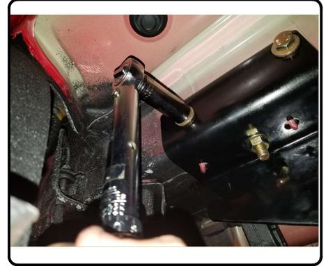
6. Torque all M10 hardware to 45 ft-lbs. and all 7/16" hardware to 59 ft-lbs. Reinstall following steps 1 and 2 in reverse order.
