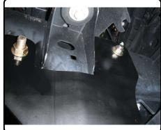
5. Torque all 1/2" fasteners to 110 lb-ft and all 5/8" fasteners to 180 lb-ft.
