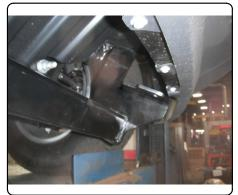
4. Pull the fishwires so the bolts hold the hitch, remove the fishwires, and loosely install the 1/2" hex flange nuts. Reinstall the tow hook bolts removed in step 1, capturing the hitch as well.
