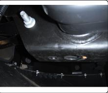
2. Fishwire the 1/2" carriage bolts and spacers into position through either the side of the frame, the end of frame, or the opening in the bottom of the frame. Do not pull bolts out through the frame so as to allow the hitch to move into position.
