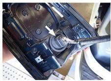
On the driver side of the vehicle, route the yellow wire up from the bottom up to the taillight cavity using a fishwire. Install the custom wiring harness with the yellow wire inbetween the factory harness.
