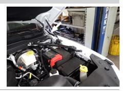
Route the 4-flat along the driver-side inner fender and mount it in the front of the vehicle under the hood.
