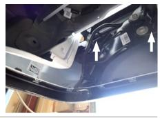
Locate a grounding point such as an existing screw or bolt in the frame of the vehicle or drill a 3/32"pilot hole. The area should be free from rust, dirt, and paint (abrasive pad/paper to remove rust and paint). Secure the white ground wire with the ring terminal on the existing fastener or with the provided ground screw.
