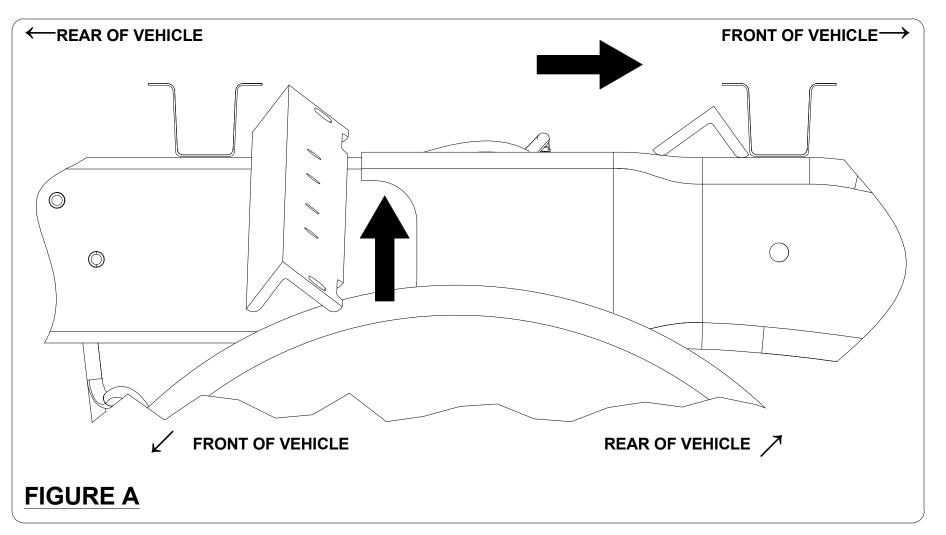
into position. The cross arm can be used as a lever to add additional bend to the flange, if needed. Insert the cross arm in the location shown in FIGURE A until it spans the frame rails. Slide the cross arm forward so that it is next to the forward bed support.
