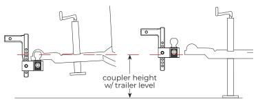
Figure 2 - Ball mount drops with added trailer tongue weight.
