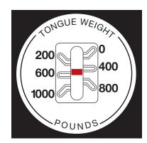
Figure 5 - Scale indicates a tongue weight of 500 lb.
