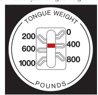
Figure 4 - Scale indicates a tongue weight of 400 lb.
