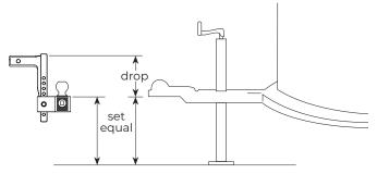
Figure 1 - With the trailer level, set the top of the ball holder at equal height to the bottom of the coupler socket.
