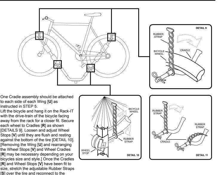
necessary with the wheel sandwiched at the end of the Pegs of the away from the Wing [**U**] [DETAIL 11]. Note: Bike Tire can be adjusted in and out to remove contact with the Rack-IT. The pads should be positioned as necessary for added protection to the finish of the bicycle.
