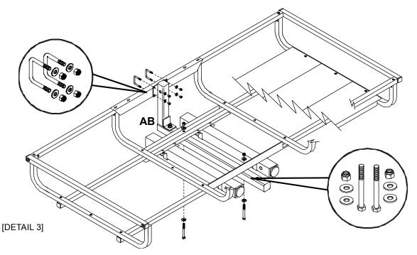
Use the remaining hardware to attach the horizontal pipe/vertical pipe assembly [A,B] as shown. [DETAIL 3]
