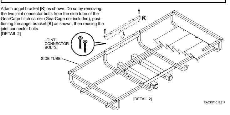
STEP 3 TOOLS: 10mm SOCKET WRENCH, 13mm SOCKET WRENCH, 13mm WRENCH
