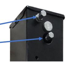
Up body hose is attached to extend port "raising" on hydraulic jack.
