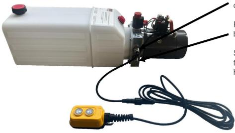
Port A – Extend / Fluid flow out of HPU
