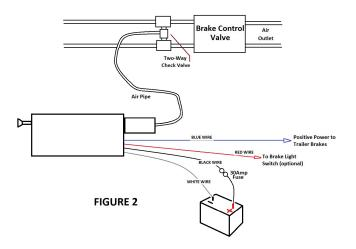
**NOTE:** The above diagram shows the two-way check valve installed in a dual air system to actuate the Hayes Brake Controller Company controller. On older vehicles with a single air brake system, the controller should be connected from the service line through a check valve to the controller.
