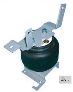
2. There are driver and passenger side units. Attach the air spring to the inboard holes of the lower bracket with the vertical flange of the upper bracket outboard. (fig. 4)
