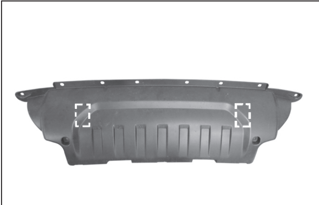
(Fig 15) Trim the approximate area to clear the Mounting Brackets through the splash guard
