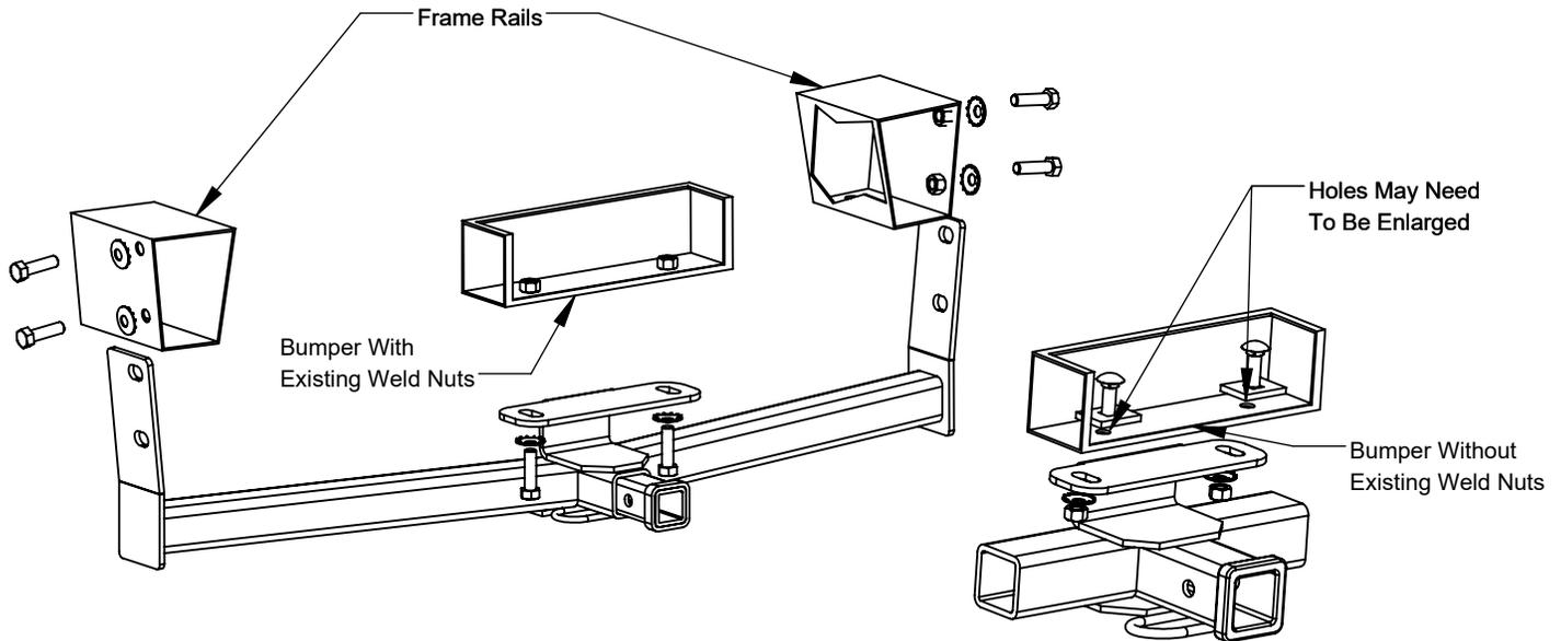
1. If present remove the tie down brackets from the frame rail. Return bolts and brackets to owner.
