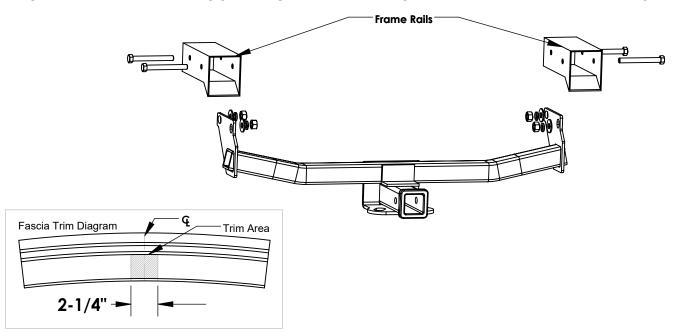
**Note:** Compass Rallye, trim out a 2-1/4" wide section of fascia centered on the vehicle up to the cross hatch pattern on the fascia. The hitch will be behind the fascia. The cutout is to allow clearance for ball mounts. Get owner's permission before cutting.
