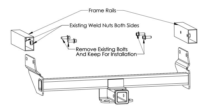
**Note:** Hitch uses existing hardware located on the vehicle for installation. No other hardware is required or included with this hitch.
