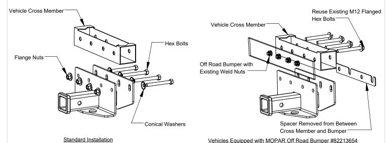
**Note:** If the vehicle is equipped with an OEM tow hook, the tow hook must be removed and returned to the vehicle owner.
